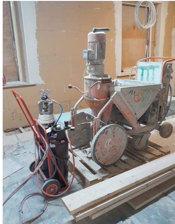
Figure 56: Plaster spraying machine
