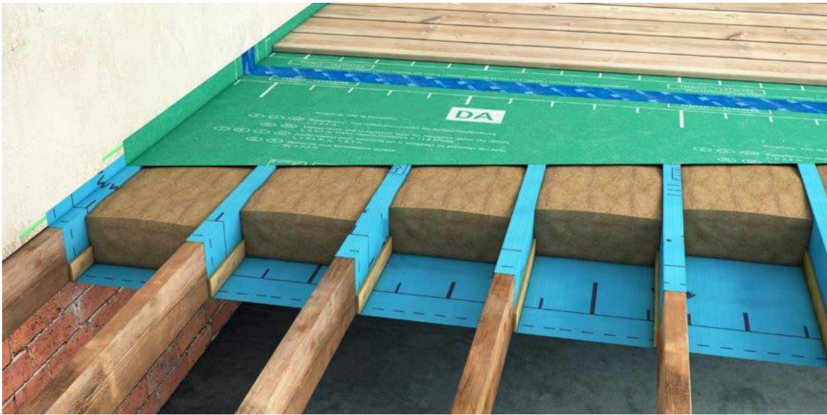
Figure 40: Slightly oversized batts of hemp insulation fit between joists over a wind-tight vapour-permeable membrane (blue) and beneath the intelligent vapour-control membrane (green). The vapour control membrane should be sealed to wall all round underneath the skirting. The solum should be cross-ventilated in accordance with TGD F and all pipework appropriately insulated
